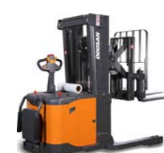
Platform Reach Stacker Pantograph Type 1.4T 24V BSR14NP
