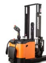
Platform Reach Stacker Mast Moving Type 1.3T-1.5T 24V BSR13/15NR
